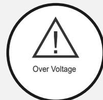
Power supply source voltage is too high, so the charger stops charging to keep your EV safe.
