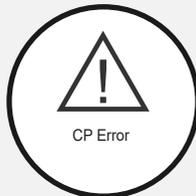
Communication error between the vehicle and charger has occurred.
